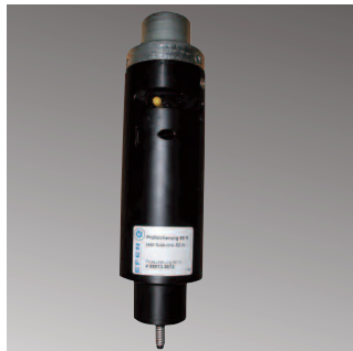
Test device for tripping device
